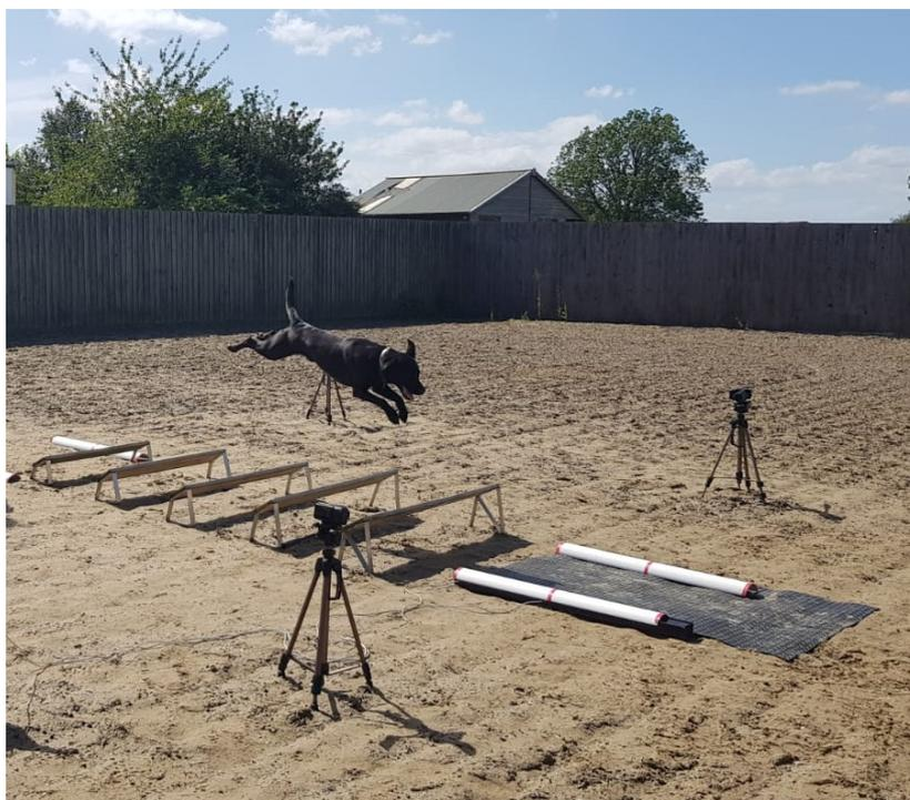
**Figure 1.** Long jump study setup showing the positioning of pressure sensing mat (under protective rubber sheeting) on the landing side.
